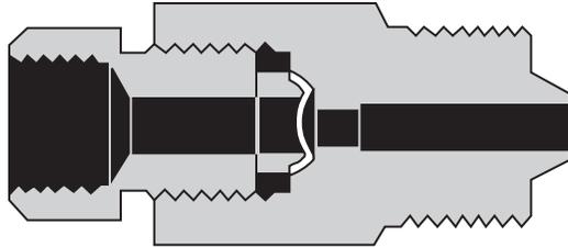
A choice of three safety head designs is available, male inlet, female inlet (straight), and tee type. The male inlet design can be inserted directly into the tubing connections of valves and various fittings such as tees and crosses, or located in pressure vessels.
